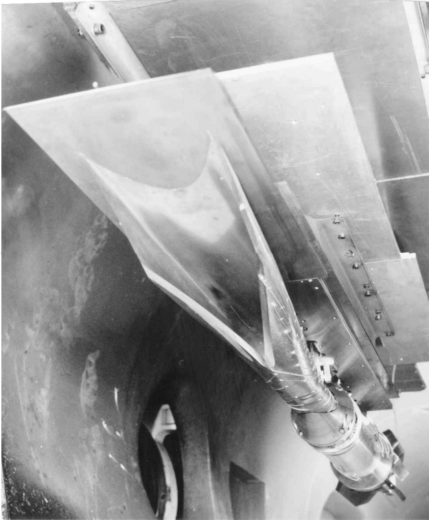
Fig. 2 Photograph of the fully assembled REST inlet model in the AHSTF test section.
